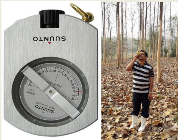
Figure 2.2. Total Tree height was measured by hypsometer, used instrument is shown in left side
